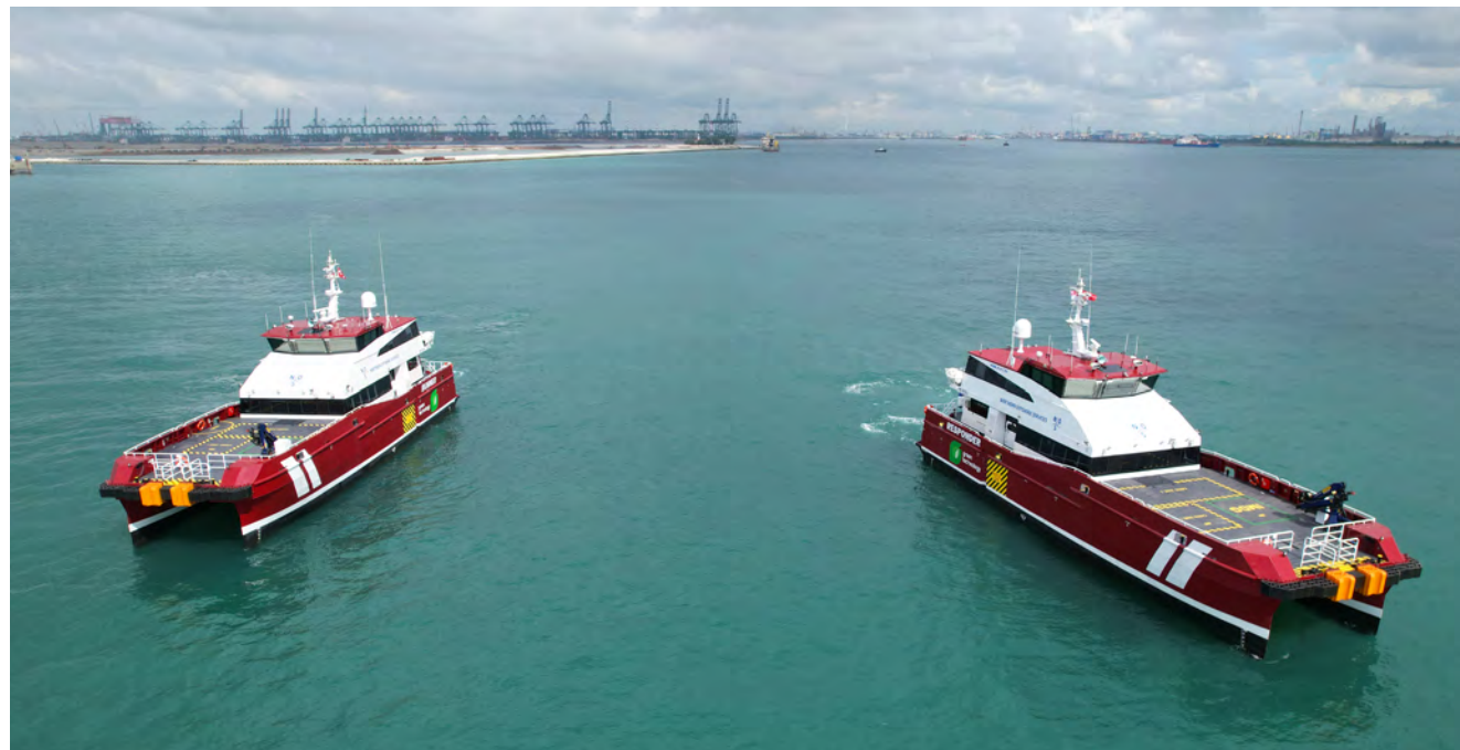
A pair of 32m hybrid-electric CTV undergoing sea trials.
