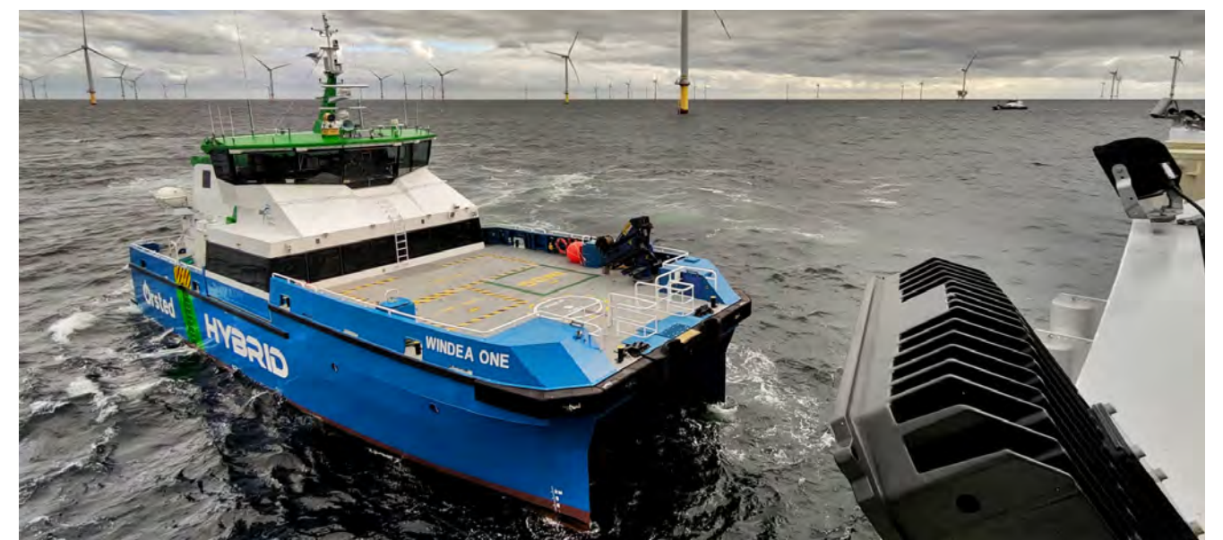
A 32m hybrid-electric CTV operating at a European wind farm.
