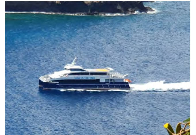
A 35m, 316-pax HSC Code catamaran ferry operating in the French West Indies.
