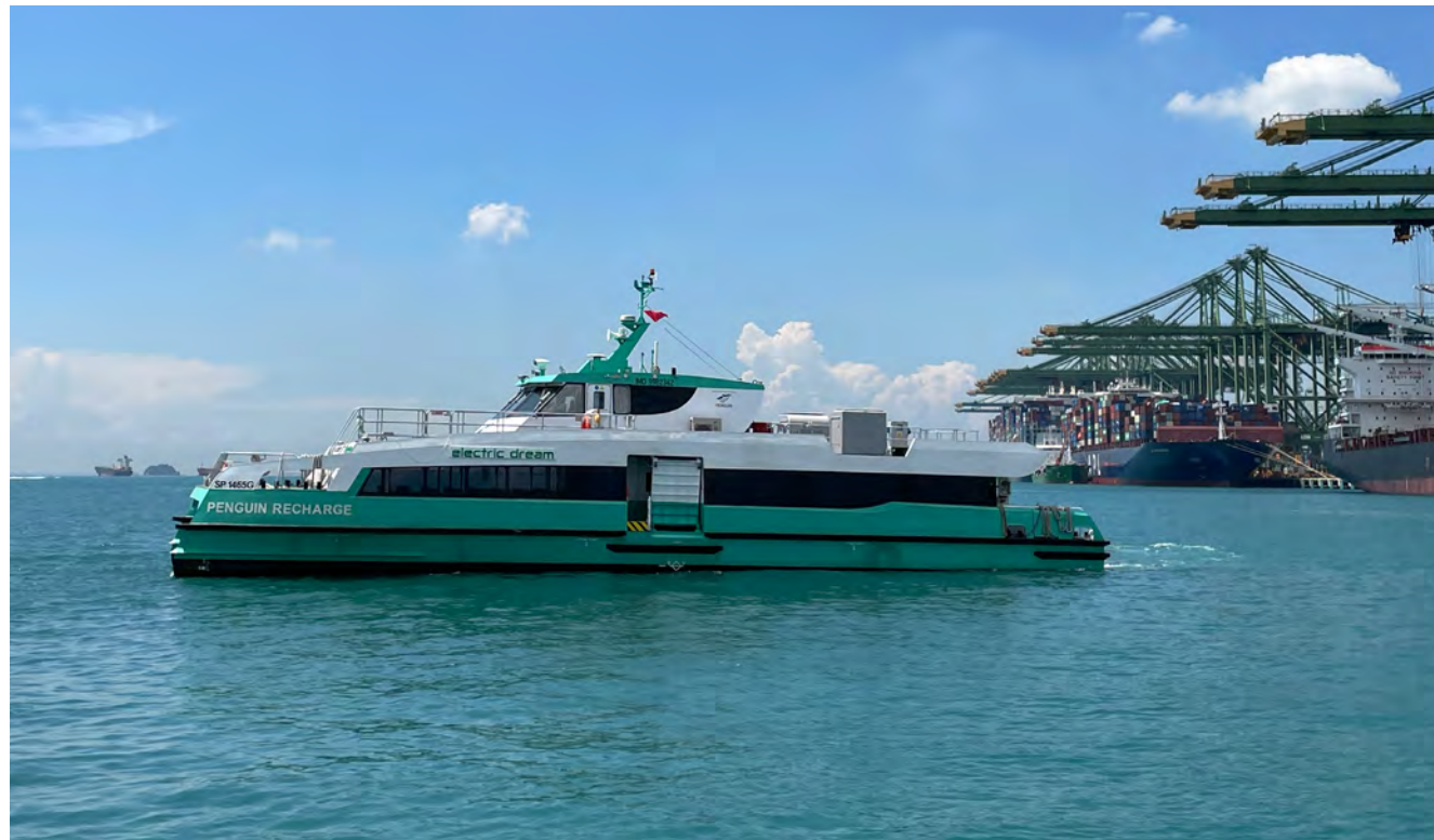
"Penguin Recharge": Cruising at 21 knots and recharging in 8 minutes.
