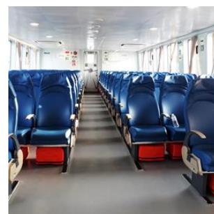
Foldable buckle-type life jacket foldable under receptacles under each seat
